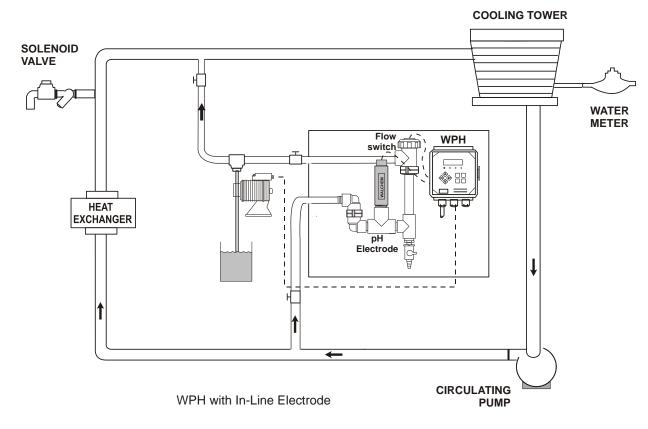
Figure 1 Typical Installation
