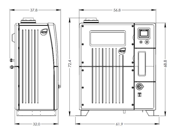
REFERENCE GENERAL ARRANGEMENT DRAWING 112-00023 FOR INSTALLATION REQUIREMENTS
