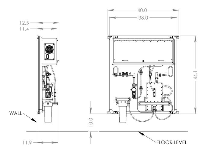
REFERENCE GENERAL ARRANGEMENT DRAWING 112-00021 FOR INSTALLATION REQUIREMENTS
